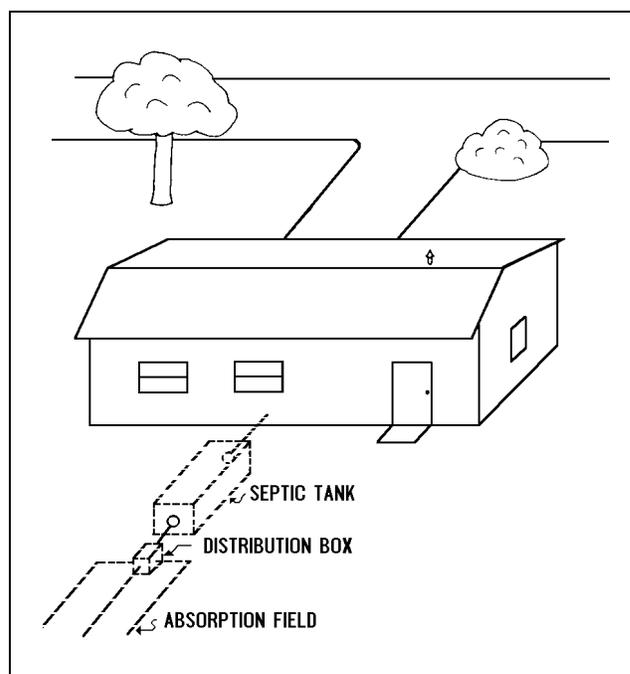
Figure 1. A typical septic system.
